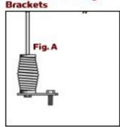
The Hydrafinder™ is adaptable to most standard fire hydrants with an easy to install 5/8" diameter bolt-on steel "flat" (Fig. A) or "L" (Fig. B) mounting bracket.
