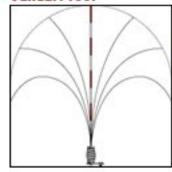
The resilient 3/8" diameter white laminar matrix fiberglass Hydrafinder™ shaft is attached to a heavy duty MIL SPEC zinc plated carbon steel spring mount that allows for 360 degree total flexibility.
